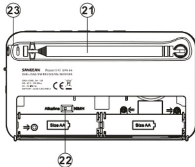
22. NiMH/Alkaline batteries switch
